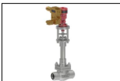
Cryogenic hydraulically actuated globe valve with butt weld ends and 300mm extension.
