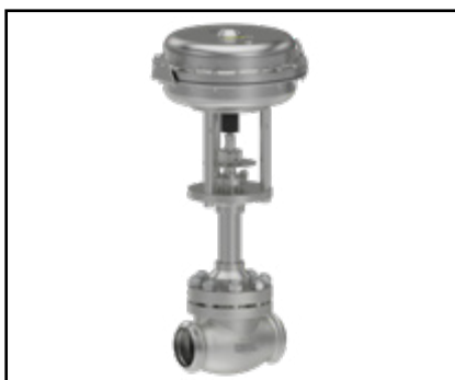
Cryogenic pneumatically actuated globe valve in DN80 size with butt weld ends, 300mm extension, and 410mm actuator, fail-close.
