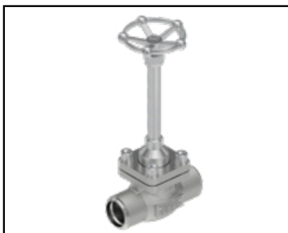
Cryogenic SDNR valve in DN40 size with butt weld ends and 300mm extension.
