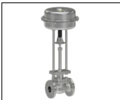
Cryogenic pneumatically actuated globe valve in DN40 size with flanged ends, 300mm extension, and 310mm actuator, fail-close.
