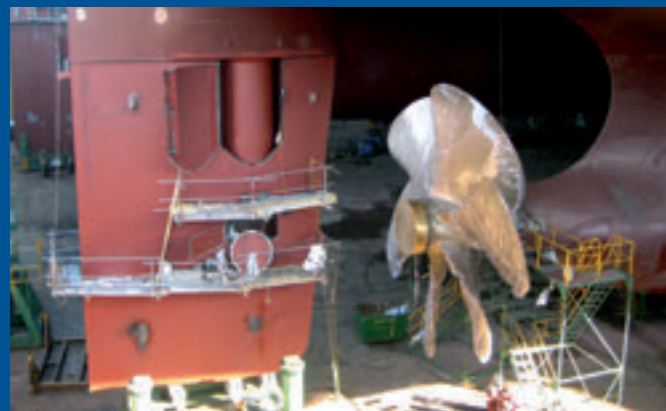
Installation of a Becker Twist Rudder with KSR
