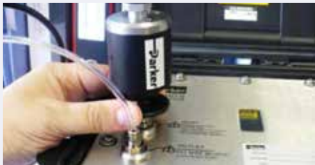
To remove the PRV, press down on the removal tool at the same time as lifting PRV off.
