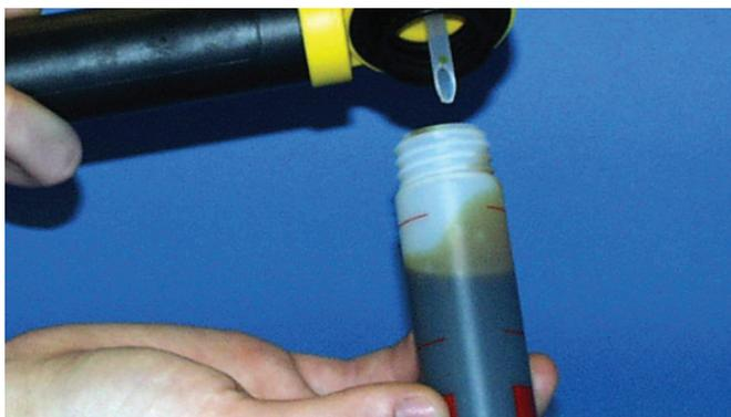
Effective predictive and preventative maintenance programs rely on scheduled oil sampling and analysis programs to provide an accurate indication of equipment and lubricant condition.
