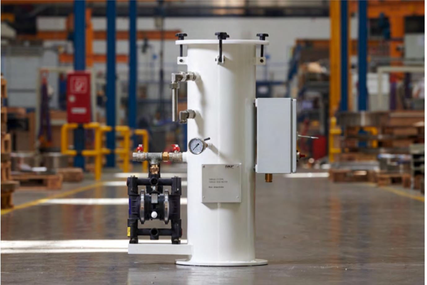
After the Turbulo Sludge Buoy's installation, the Turbulo SolidMaster serves as filtration system which precedes the oily water separator (OWS) and mechanically removes suspended solids in the bilge water. Doing this before running the bilge water through the separator helps avoid the formation of suspensions and thereby extends the lifetime of the – more expensive – separation elements of the OWS.
